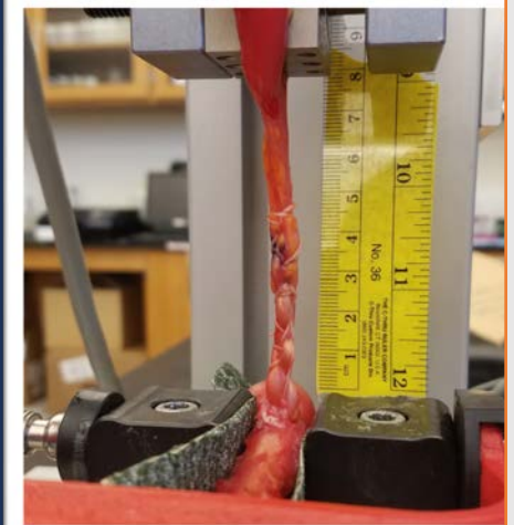
Image 3: Assessing gapping after cyclic loading
