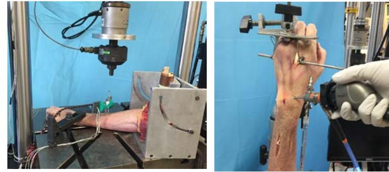
A) Specimen mounted with optical trackers attached to pelvic screws inserted in radius and ulna. Instron ram loaded ulna with 5 cycles +/-40 Newtons.
