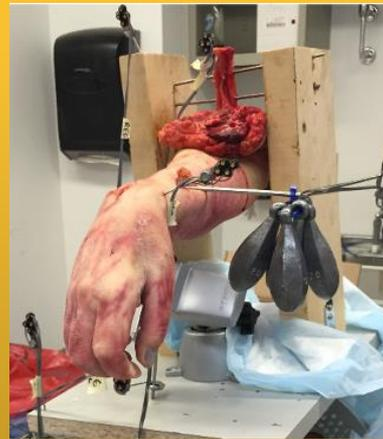
Figure 1 illustrates a cadaveric specimen in the experimental jig undergoing 4 Nm of pronation torque. Note the LED markers attached to the radius, ulna, humerus, jig base, and right jig tower.
