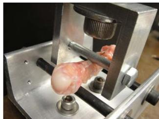
3-Point Bending Apparatus
