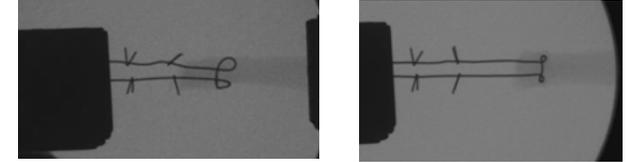
Figure 6. Deformation of simple loop link component, before (left) and after (right).
