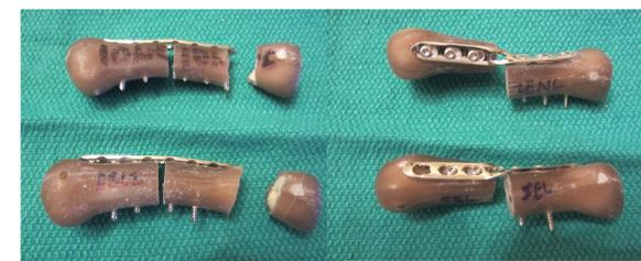
Figure 2. Failure modes for cantilever bending (Left) and torsion (Right). Nonlocked constructs are above and the locked constructs are below.
