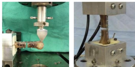
Figure 1. Testing apparatus for cantilever bending (Left) and torsion (Right).
